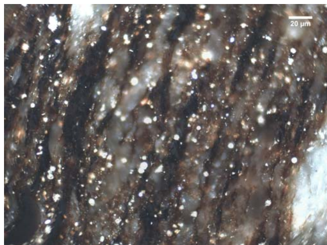
Figure 8. Generic examples of bituminite. Oil immersion, reflected white light
