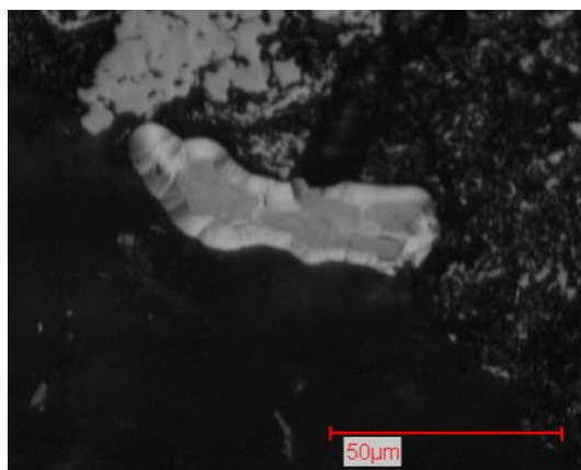
Figure 3. Pyrolytic carbon in coal waste dump. Portugal, metaanthracite waste pile, R_r = 4.10 - 6.25\% . Polarised incident white light.
