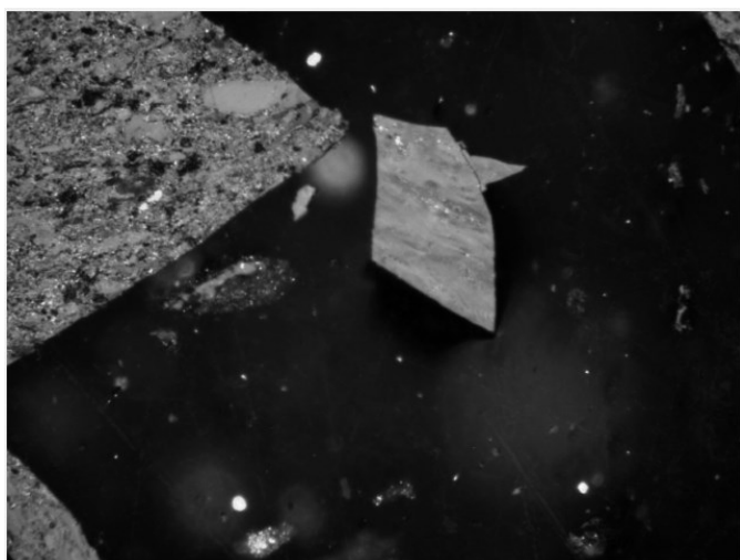
Fig 1 (L): A good looking field of view but an air bubble is present in the oil which would affect reflectance measurements
