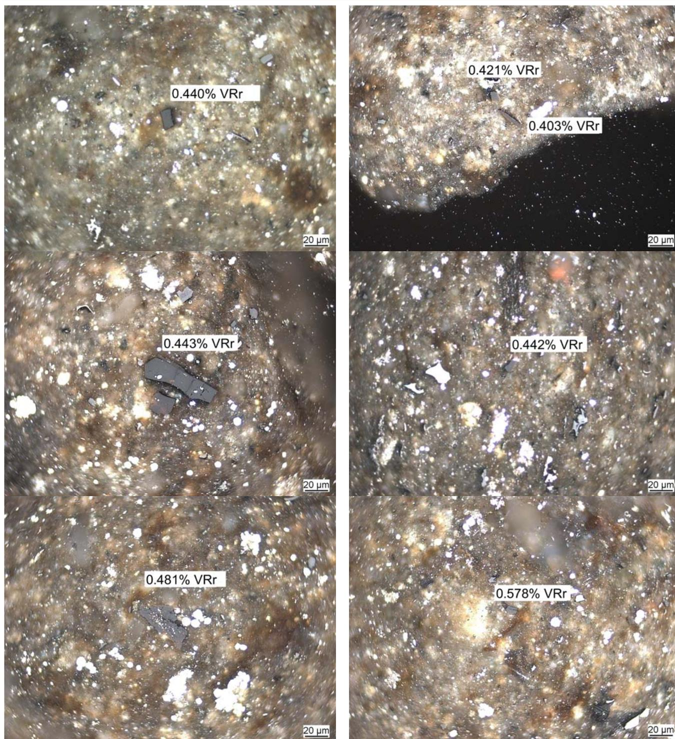
Fig. 5. Photomicrographs of vitrinite particles in whole rock sample allocated either to the first or the second vitrinite population. Magnification 500 X; oil immersion objective.
