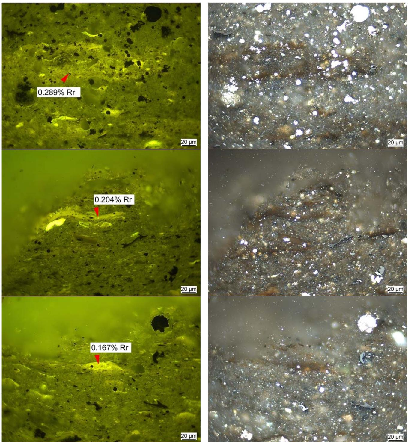
Fig. 10. Photomicrographs of bituminite particles in whole rock sample. Magnification 500 X; oil immersion objective.
