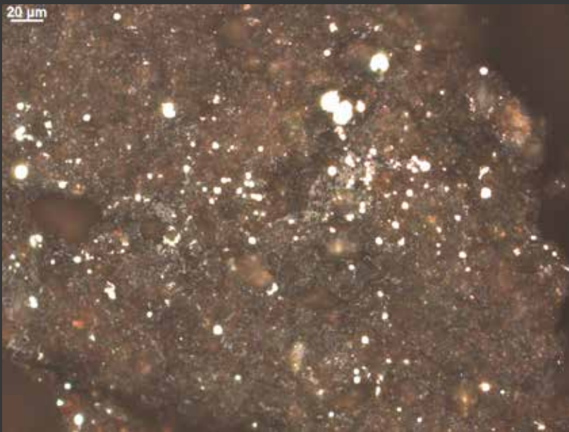
Jurassic shale from important North American shale gas play: TOC 2.66 wt.%, R_o > 1.0\%
